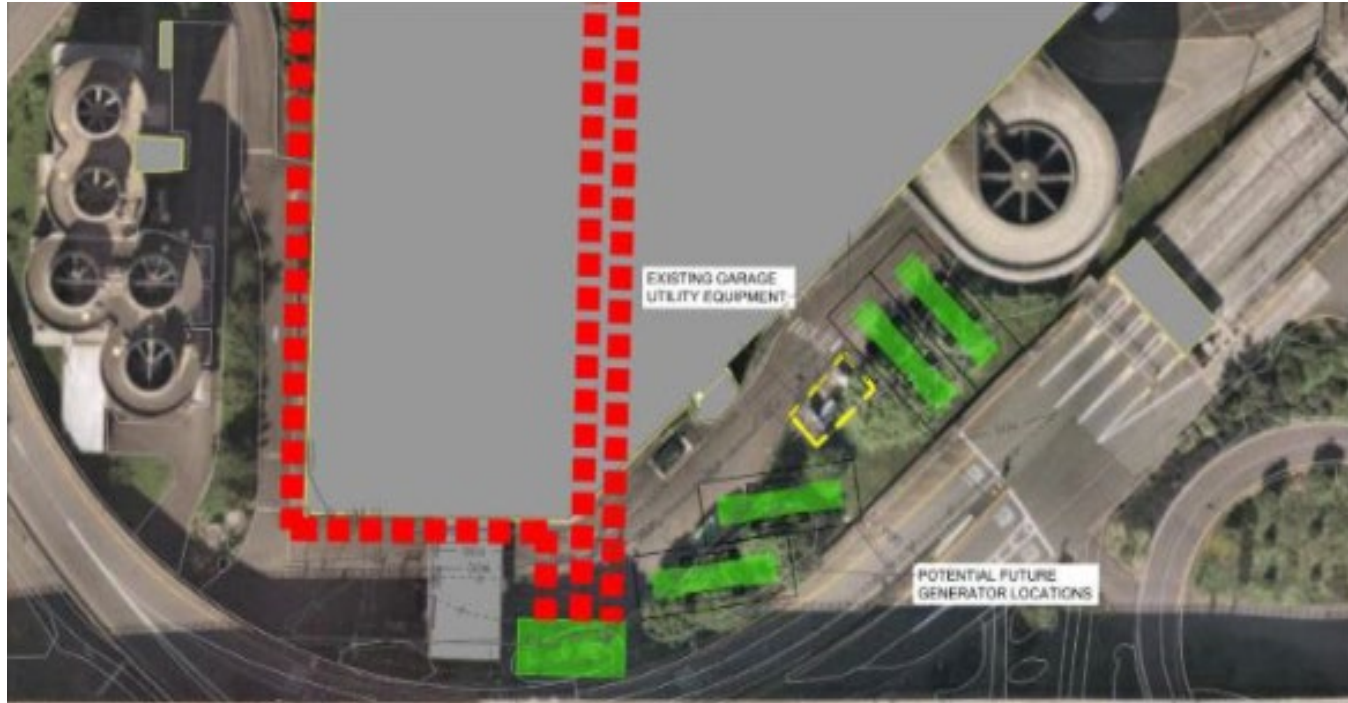
Southern edge of the garage, with potential generator routes shown in red dash.
