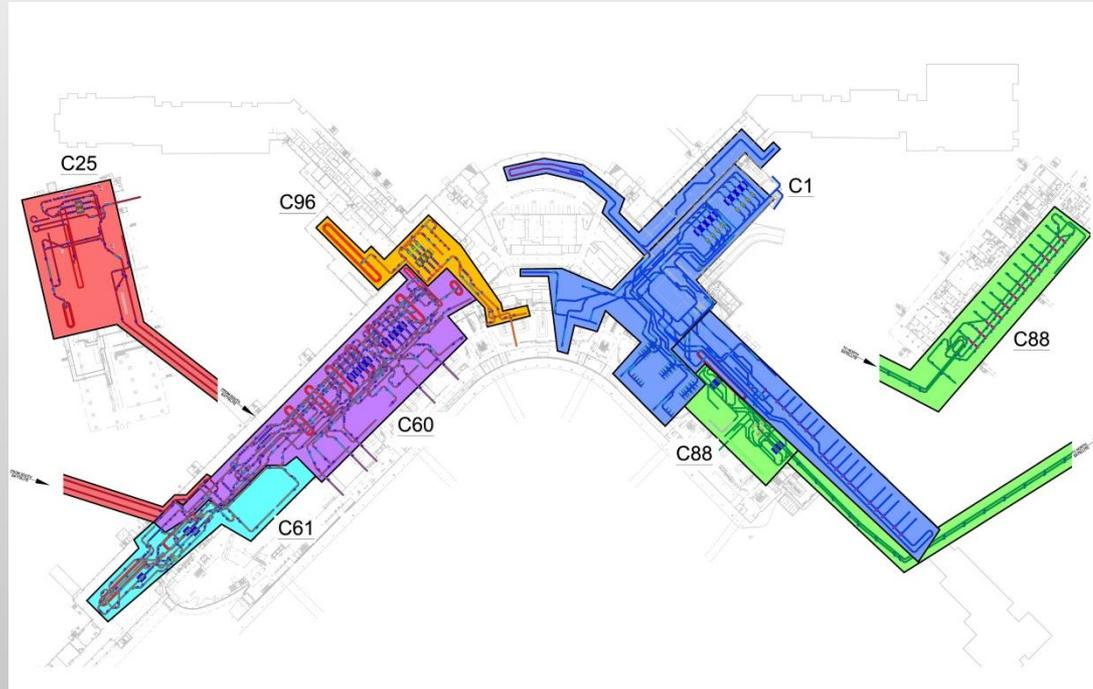
Current baggage handling system has six separate outbound systems.
